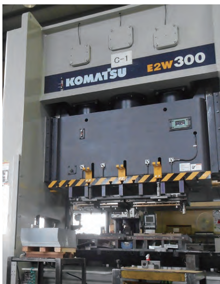
当社所有の最大加圧能力の300tプレス機 Our greatest pressing machine able to exert up to 300 t
