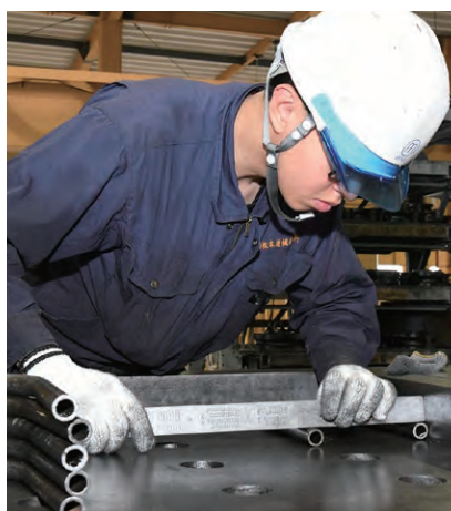
パイプの両端の幅を測り、寸法を確認 Dimensional check by measuring the width of both ends of a pipe
