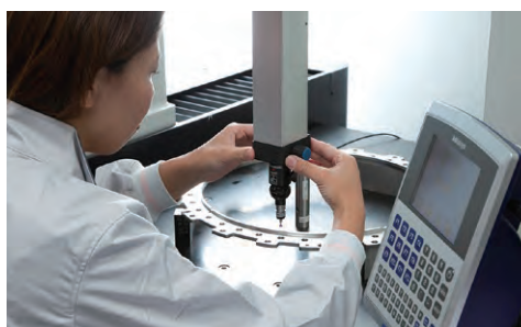
三次元測定機による検査風景 Testing with a three-dimensional measuring machine
